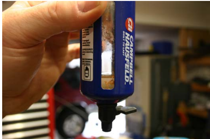
Figure 4 – One compressor cycle worth of removed water
