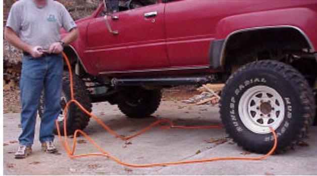
The key part for this cheap trick is a Schrader valve to nominal pipe thread (NPT) fitting. With this, you can use any ordinary tire chuck to pressurize a system, or an ordinary tire pressure gauge to check all 4 tires at once.
