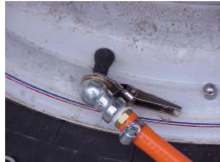
You will need four locking type tire chucks, shown here. These lock onto your tire's valve stem so you dont have to hold them. If you have on-board air in your vehicle, you install one of these and stand back and watch all four tires air up at the end of the trail.
