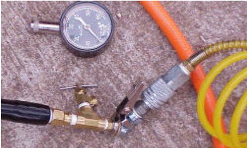
Airing back up is just reconnecting the deflator and either holding a service station tire chuck onto the deflator (boring), or else connecting your locking chuck from your onboard air (cool). Here is a locking tire chuck from my compressor hooked up re-inflating all four tires.
