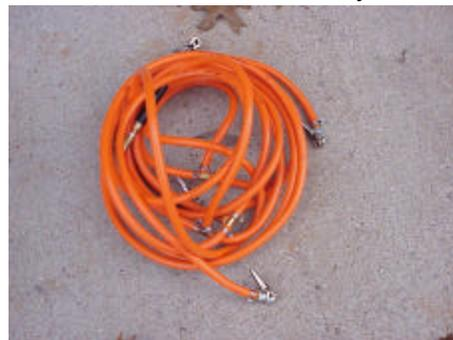
around all four tires in a sort of loop and fill from one end. The whole thing ends up taking up about 1 square foot by three inches thick when rolled up. I found an old cloth bag to keep it in.
